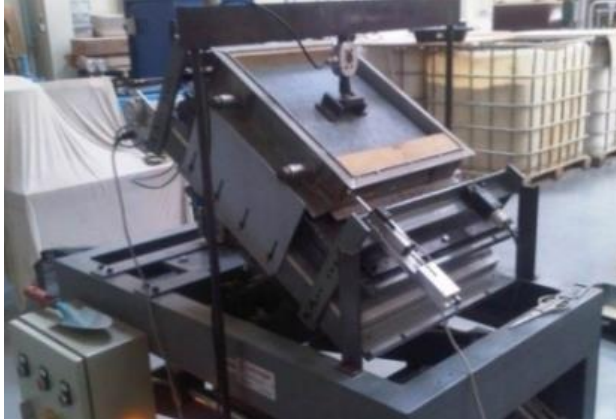
Figure 2 – Equipment used for: a) pull-out tests; b) inclined plane shear tests.
