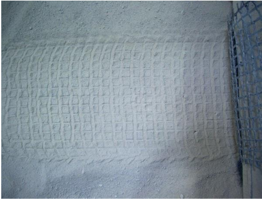
Figure 8. Negative of GGR in the confining soil (S4) after a pullout test.
