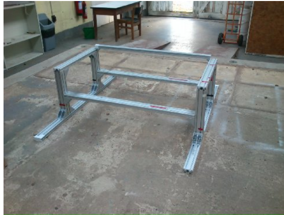
Figure 5-4 - NIMBLE actuator support frame – The actuator is suspended between the two horizontal aluminium profiles in the centre.
