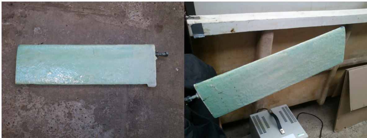
Figure 5-9 – Fibre glass reinforced NACA0012 foil build for the actuator.
