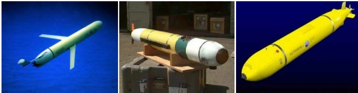
Figure 1-2 - Different types of AUVs. Slocum glider (left), Remus 100 (centre), Autosub 6000 (right). Image source: AUVAC
