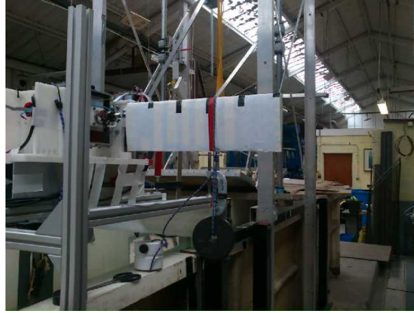
Figure 5-15 - Foil undergoing strain gauge calibration
