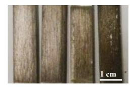
Figure 7.4 Pictures of the temperature varied Ni-P/WS<sub>2</sub> samples (from left to right: 80°C, 60°C, 40°C, and 20°C).
