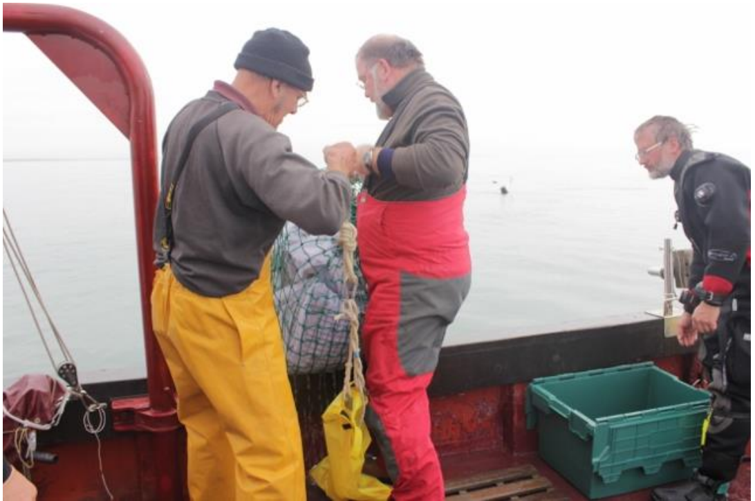
Figure 2.4 Each reef box was wrapped in a fine mesh net (white net) to prevent the escape of mobile fauna and was secured in a second mesh net (green cargo net) for the purpose of lifting it on board.
