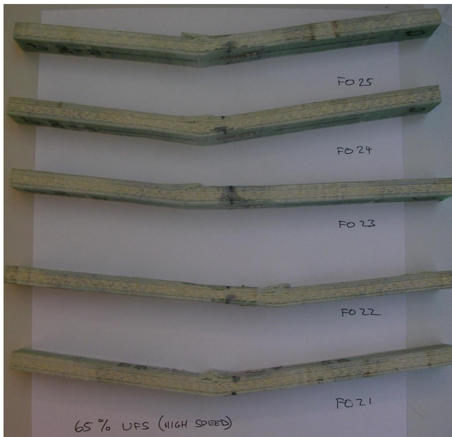
Figure 11-60: Coupons F[0]-21 to F[0]-25 tested at a strain rate of 30mm/min CCLXII
