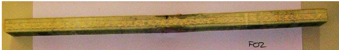
Figure 4-6: Typical post failure sample for static tests F[0]-01 to 05.
