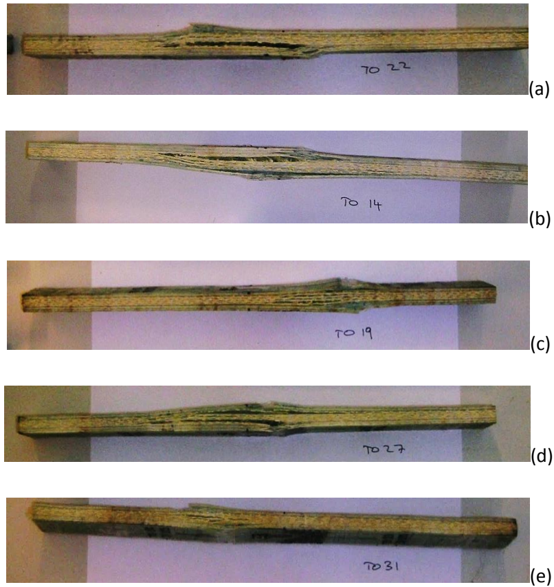
Figure 4-20: Examples of post fatigue failure modes of selected samples for each of the applied load ratios, (a) R_{app} = 0.9 , (b) R_{app} = 0.8 , (c) R_{app} = 0.7 , (d) R_{app} = 0.6 , (e) R_{app} = 0.5 .
