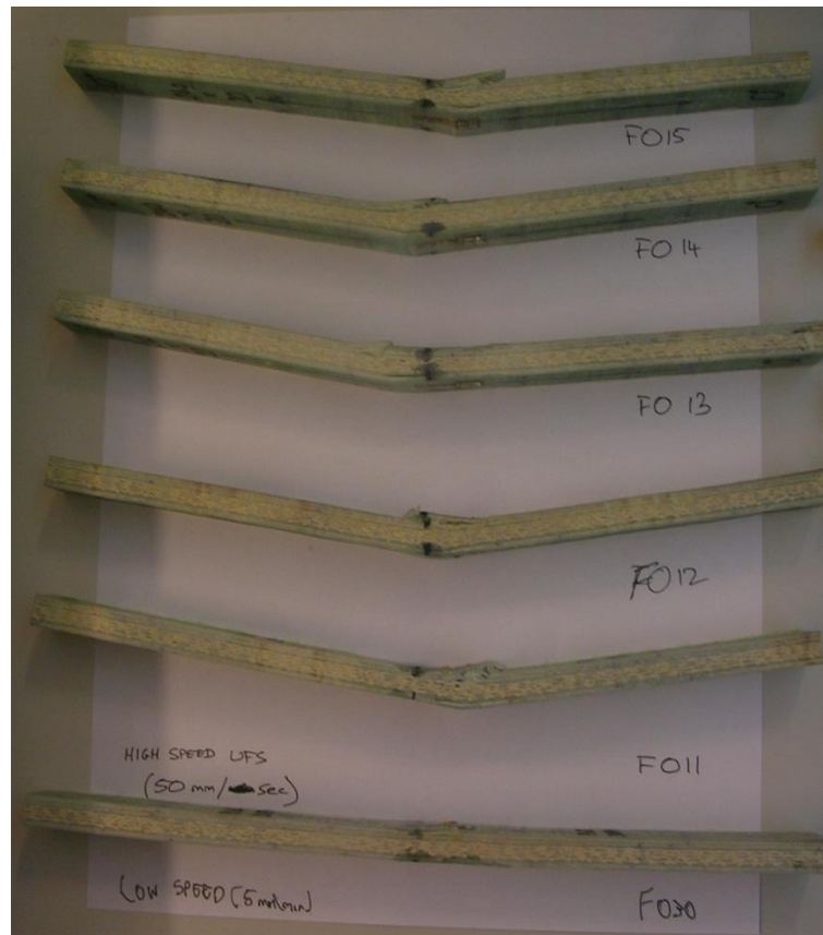
Figure 11-42: UFS results for [0] direction coupons F[0]-11 to F[0]-15 tested at a strain rate of 30mm/min
