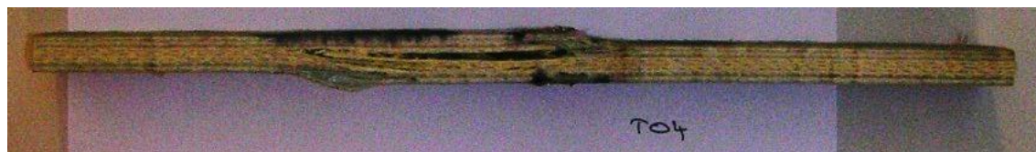
Figure 4-2: Typical post failure images for tensile tests in the [0] direction.
