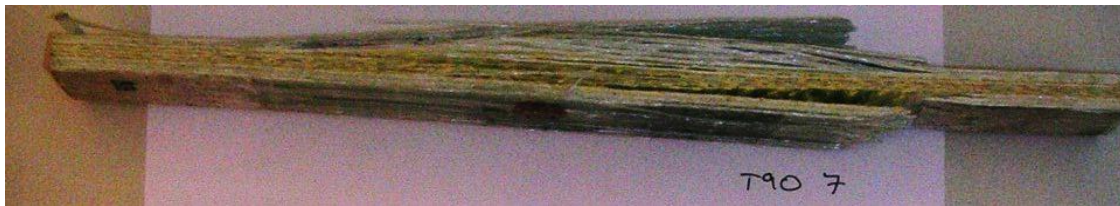
Figure 4-4: Typical post failure images for tensile tests in the [0] direction (a) and the [90] direction (b)
