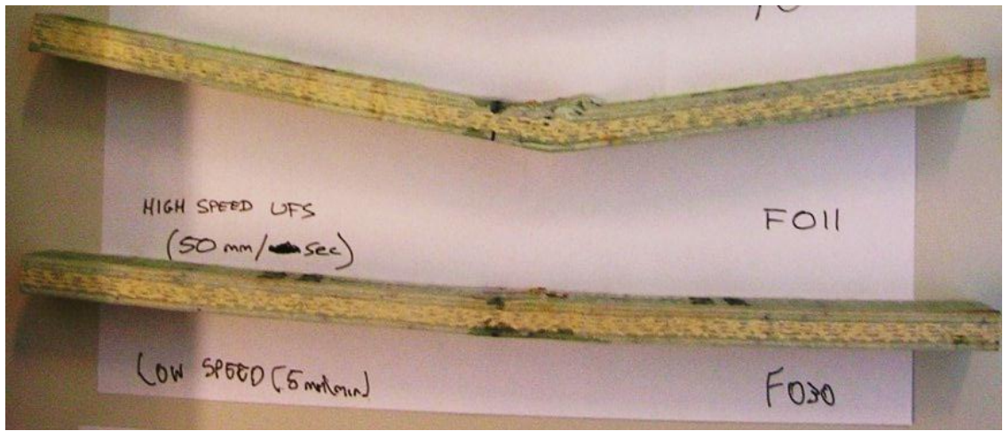
Figure 4-9: Typical post failure sample for static tests F[0]-011 to 15 and F[0]-30.
