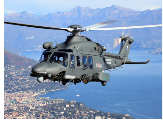
(b) Semi-retractable-wheel undercarriage (AW139M), AgustaWestland (2015).
