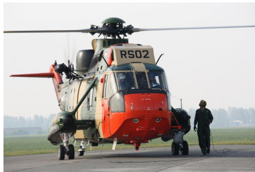
(b) Hull shaped fuselage of the Westland SeaKing Mk48, Belgian Defence/DG COM.
