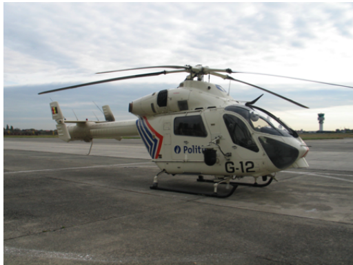
(c) Tail boom with air slots (MD-900), Terence Rayee, ULB.
