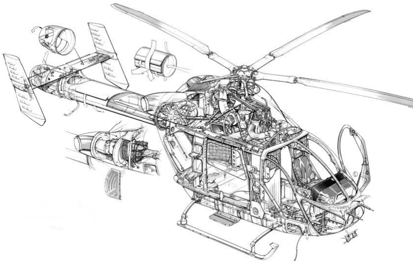
FIGURE 1.8. The internal architecture of the MD-900 with NOTAR. Note the absence of a tail boom shaft and the presence of a fan in the tail root, required to generate the compressed air flow. The size of the transmission system is clearly reduced with respect to the helicopters with tail rotor. Adopted from FlightGlobal (2015).
