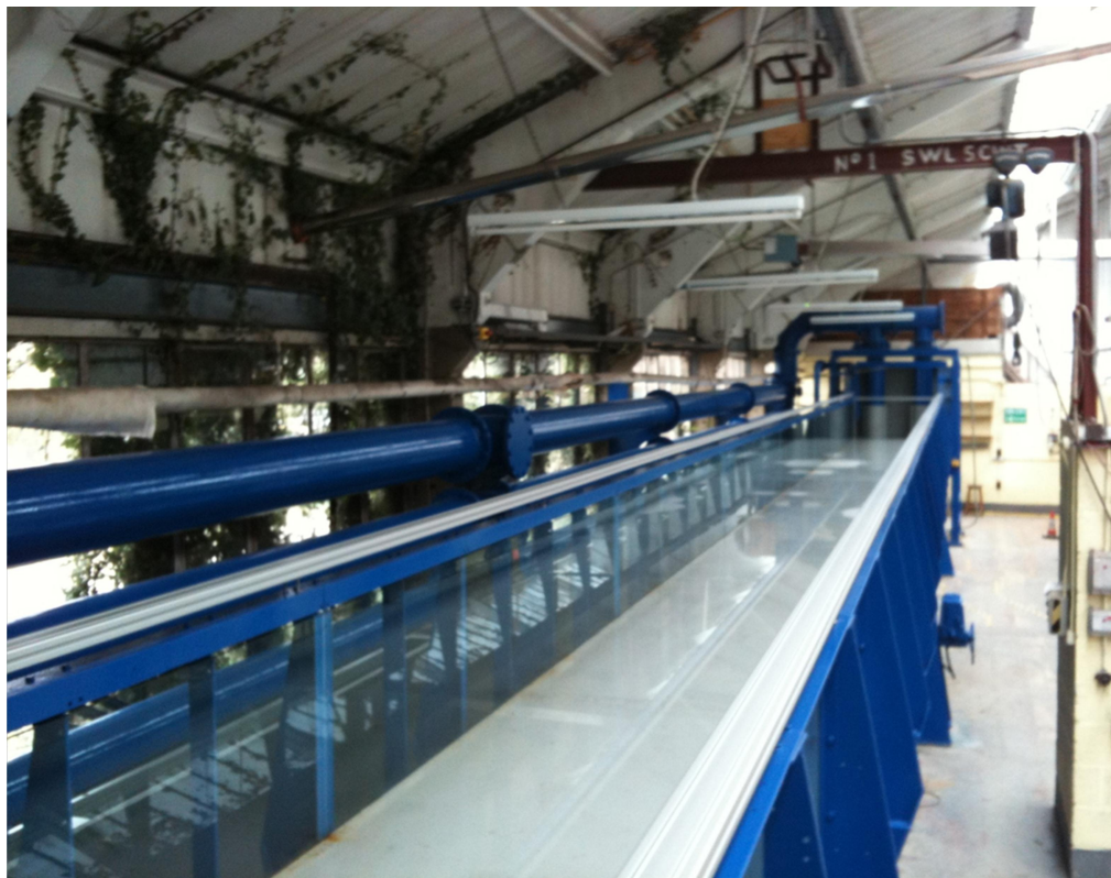
Figure 3.1: Indoor circulating water flume of Chilworth laboratory
