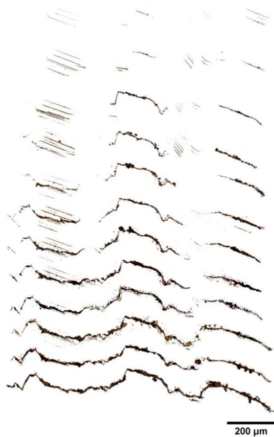
Fig. 4.5 Evolution of the primary crack in the interrupted test for the CG LSHR U-notch specimen.
