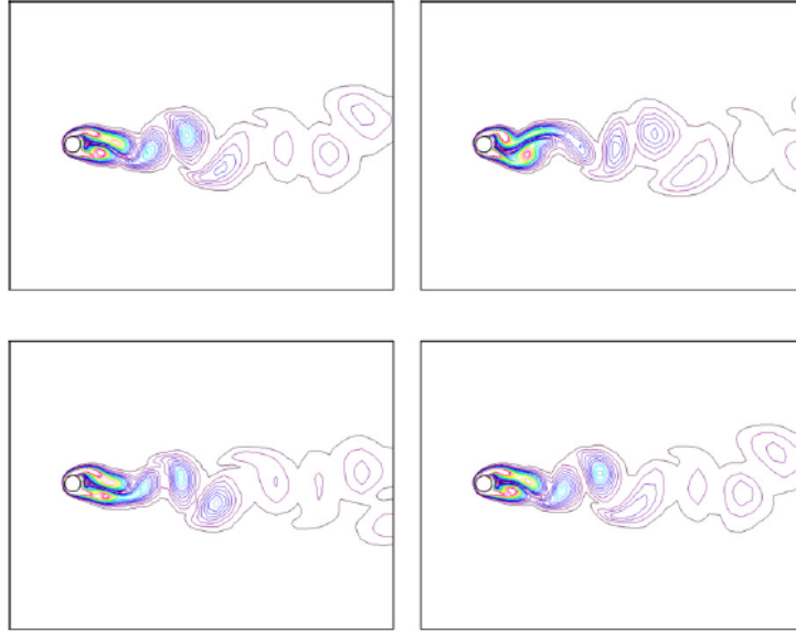
Figure 6.33: Vorticity profiles around cylinder oscillating at Re = 100 , Y = 0.25D , F = 1.5 obtained by Placzek et al. (2009)
