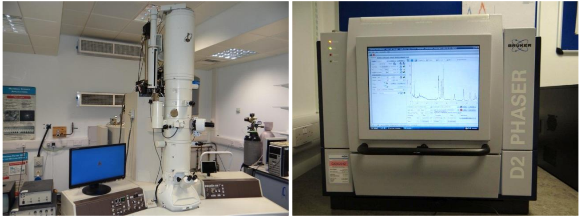
Figure 3.6: Left: the TEM microscope (JEOL JEM-3010, Japan) and right: the XRD facility (D2 Phaser, Germany) facilities used in this study.
