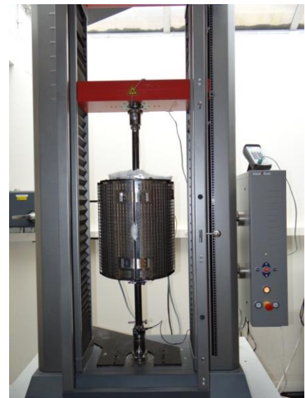
Figure 3.13: Left : Schematic illustration for the positions of tensile samples within the HPT disk [99], and right : The tensile machine (Z030, Germany) used in in this study.
