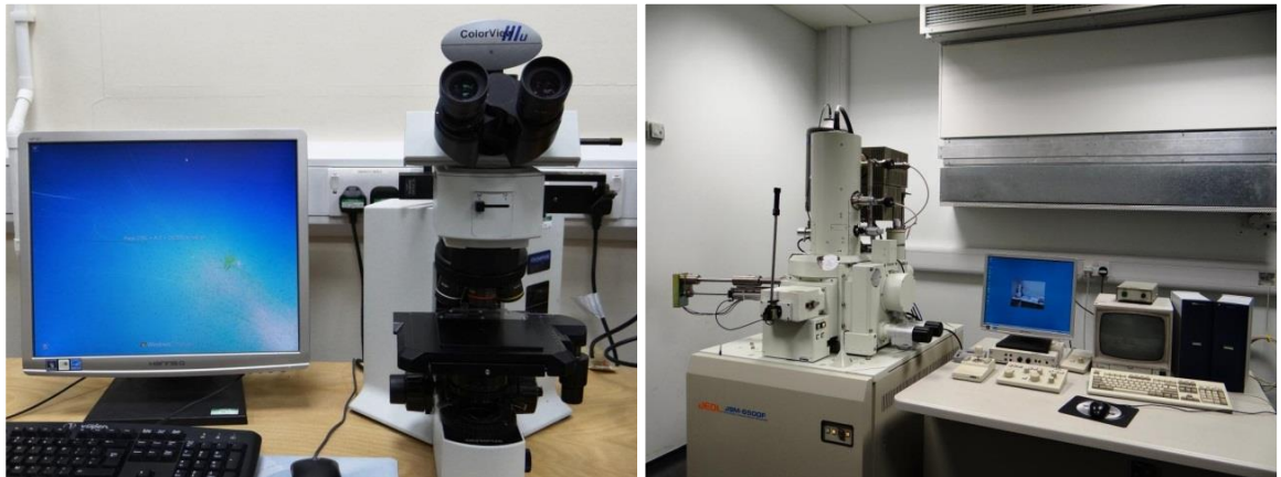
Figure 3.5: Left: the optical microscope (OLYMPUS–BX51, Japan) and right: the SEM microscope (JEOL JSM–6500F, Japan) facilities used in this study.
