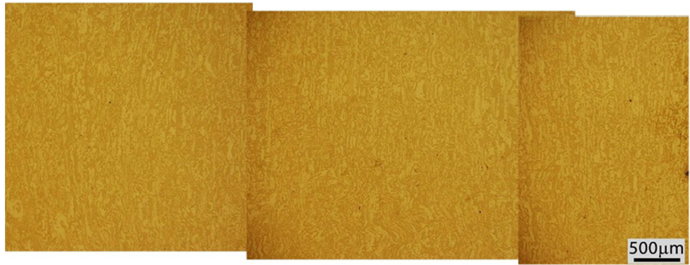
(b) Rough anvil, misalignment of 100 \mu\text{m} , N = 5 , bottom surface
