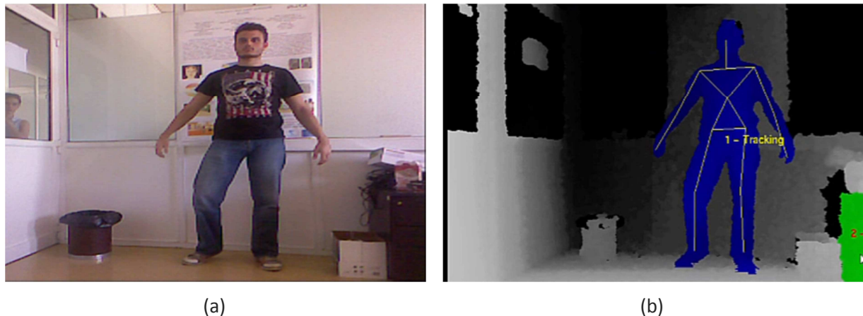
Figure 1 - Sample data captured by the Kinect for Xbox 360 sensor
