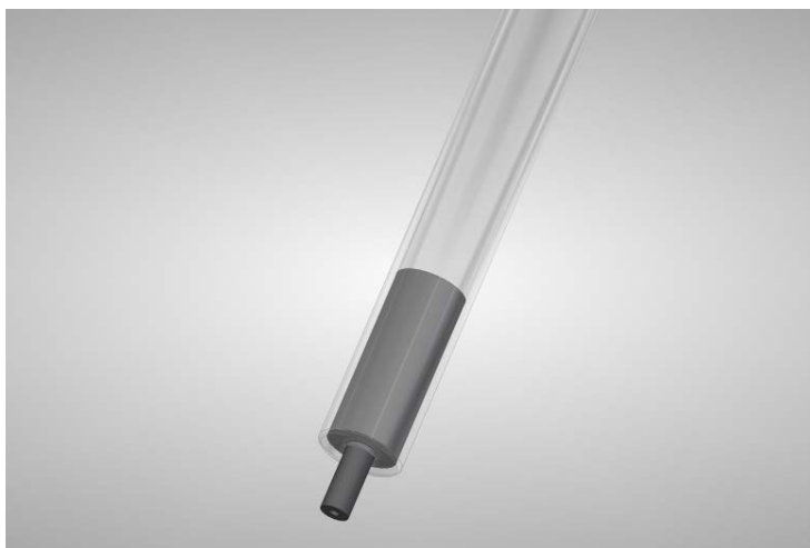
Figure 6.9 GLS crucible drawing apparatus with vitreous carbon nozzle
