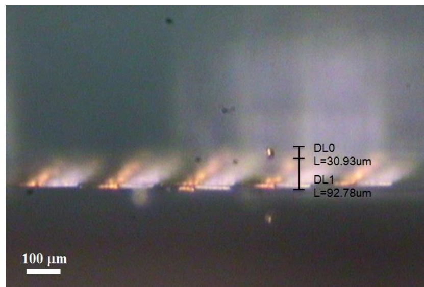
Figure 8.19 – Photograph of a single 30 \mu\text{m} glass microsphere trapped in a 2D hexagonal lattice trap at 93 \mu\text{m} above the electrode surface. The measured trap height is less than the simulated value of 117 \mu\text{m} due to a small tilt angle of the CCD side camera.
