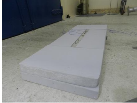
Figure 20. Sleeper embedded in melamine foam
