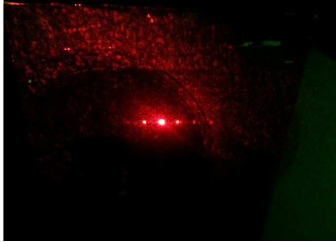
Figure 4.8: Photograph of self-diffracted beams from a typical liquid crystal light valve.
