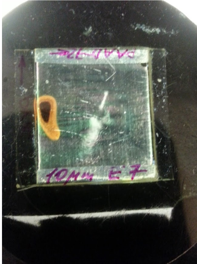
Figure 6.9: Photograph of the PAAD/PVK:C 60 cell after exposure to linearly polarized blue light. The lighter areas towards the centre of the cell indicate that the LC is in a twisted geometry in those areas, and exposure has not caused the LC to completely re-align at the PAAD/LC interface. Therefore, those areas are avoided when performing the diffraction efficiency experiment.
