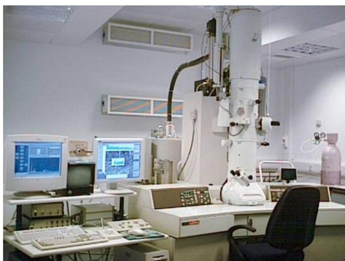
Figure 3.3 Jeol 3010 transmission electron microscope, University of Southampton [154].
