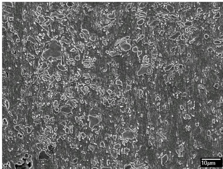
Figure 4.29 SEM micrograph (SEI mode) showing the microstructure at the edge of the FM sample (0.1 wt.% C) processed by HPT up to 4 turns and etched with 2% nital.
