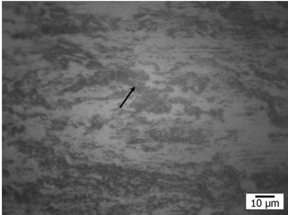
Figure 4.15 Representative optical micrograph showing the impression of one indentation in the pearlite at the edge of the FP sample processed up to 4 turns and etched with 2% nital.
