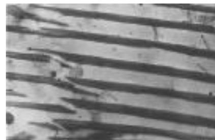
Figure 2.18 TEM bright-field image showing the lamellae structure of pearlite in low-carbon steel (0.15 mass.% C) [48].
