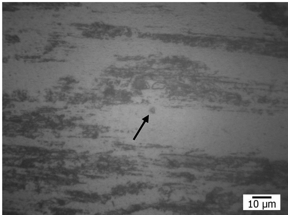
Figure 4.14 Representative optical micrograph showing the impression of one indentation in the ferrite at the edge of the FP sample processed up to 1 turn and etched with 2% nital.
