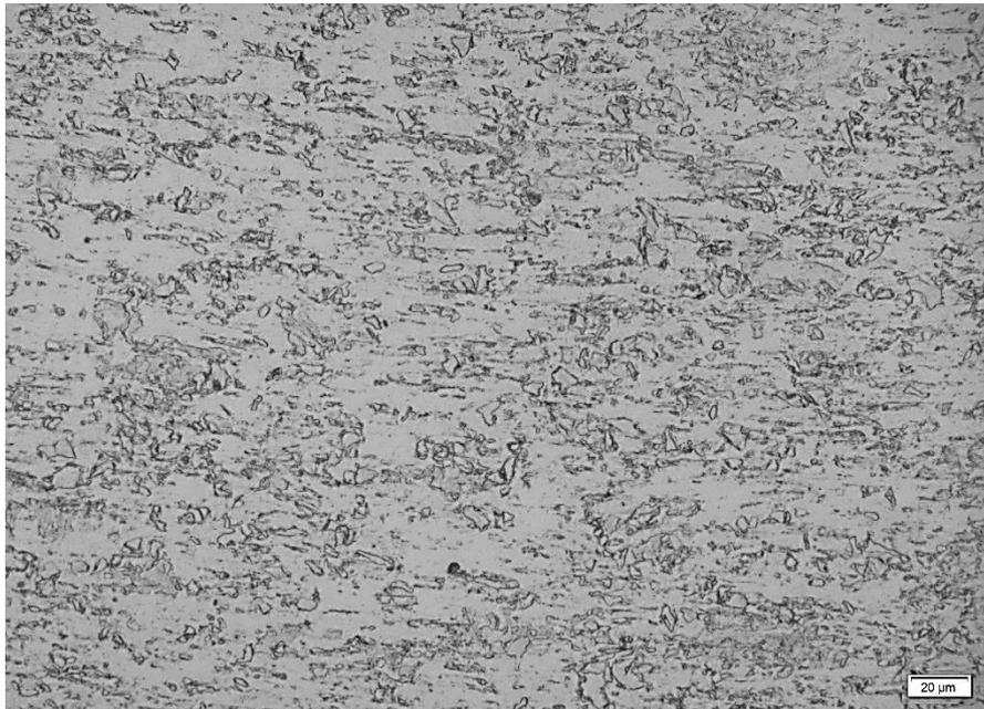
Figure 4.27 Optical micrograph showing the microstructure at the edge of the FM sample (0.1 wt.% C) processed up to 1 turn and etched with 2% nital.
