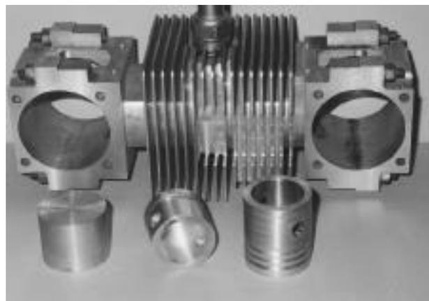
Figure 2.16 Piston manufactured from nanostructured Al 1420 alloy used in small internal combustion engine [44].
