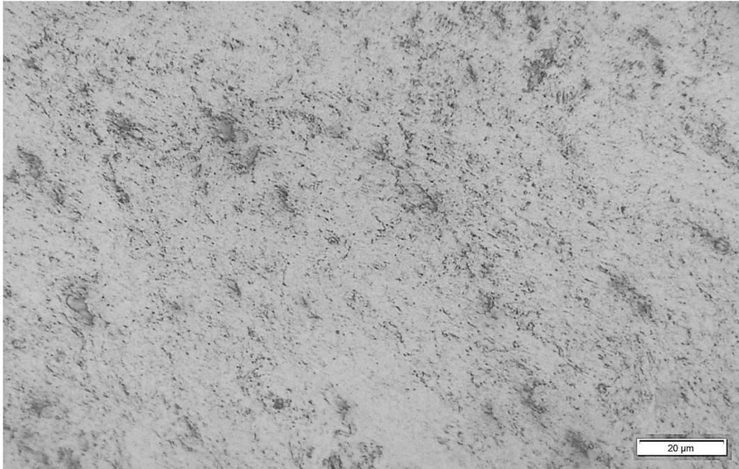
Figure 4.24 Optical micrograph showing the microstructure at the edge of the FP sample (0.1 wt.% C) processed up to 10 turns and etched with 2% nital.
