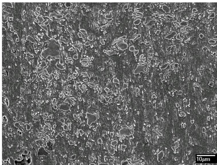
Figure 4.29 SEM micrograph (SEI mode) showing the microstructure at the edge of the FM sample (0.1 wt.% C) processed by HPT up to 4 turns and etched with 2% nital.
