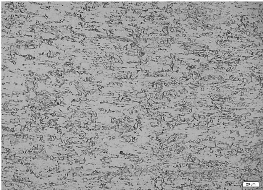
Figure 4.27 Optical micrograph showing the microstructure at the edge of the FM sample (0.1 wt.% C) processed up to 1 turn and etched with 2% nital.
