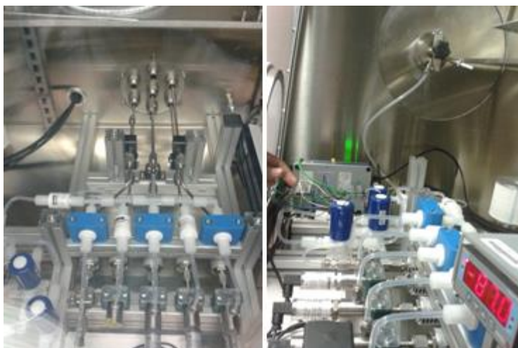
Figure 37 Pictures showing the purifier and dew point during installation within the glovebox
