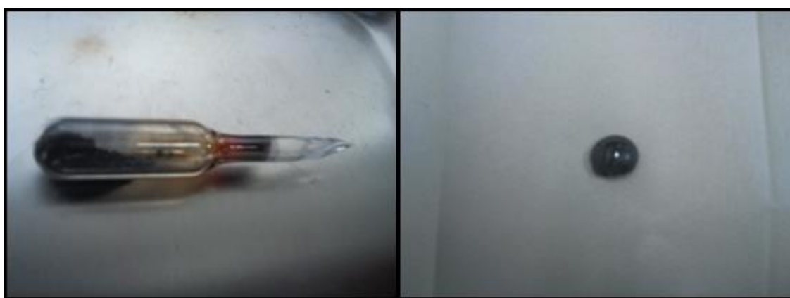
Figure 16 Result of a microwave synthesis of \text{As}_2\text{Se}_3 attempt during this work
