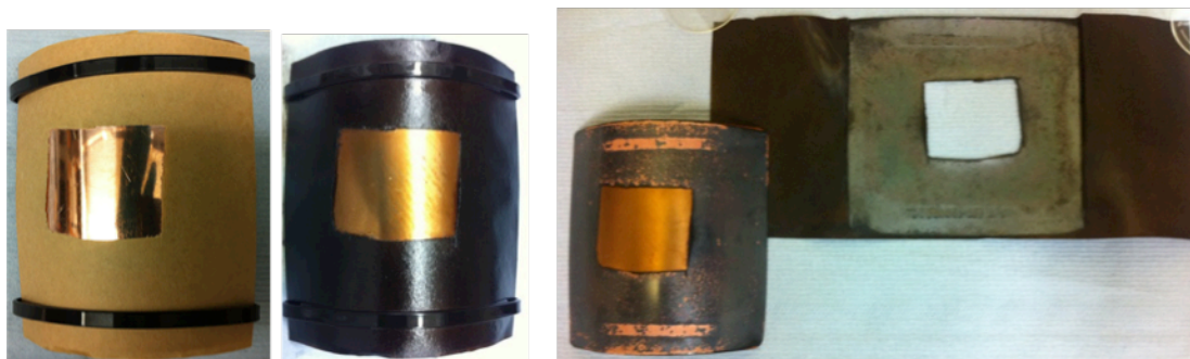
Figure 41 – Appearance of the sample before (left) and after (middle) ageing for 7 days in oil at 140 °C in the presence of air and 2000 mg kg -1 of DBDS. An overview of the status of both copper and paper is shown (right).
