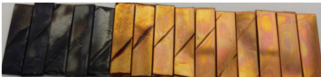
Figure A104 – Copper samples inhibited with increasing amount (left to right) of Irgamet ® 39 in HyVolt III oil after the CCD test in the presence of 2000 mg kg -1 of DBDS.
