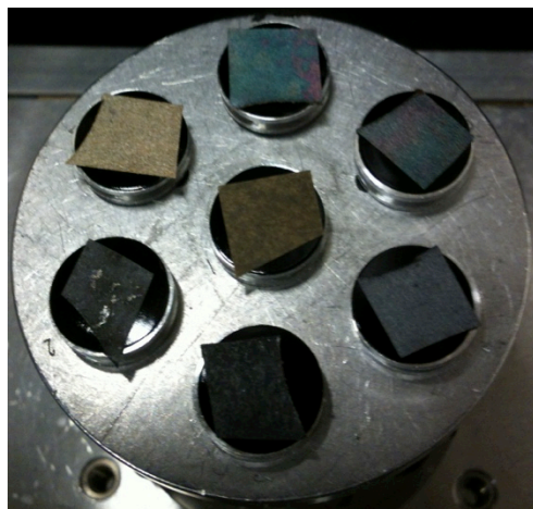
Figure 20 – Paper samples secured onto the ESEM sample holder.
