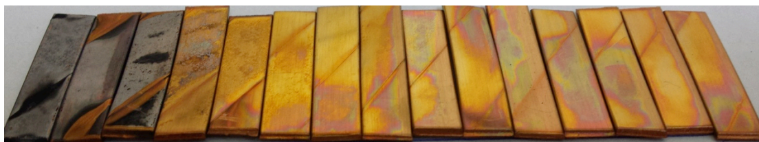
Figure A103 – Copper samples inhibited with increasing amount (left to right) of Irgamet ® 39 in Gemini X oil after the CCD test in the presence of 2000 mg kg -1 of DBDS.
