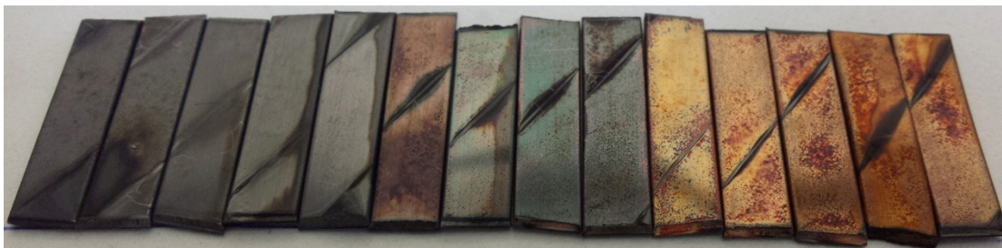
Figure A105 – Copper samples inhibited with increasing amount (left to right) of Irgamet ® 39 in 10 GBN oil after the CCD test in the presence of 2000 mg kg -1 of DBDS.
