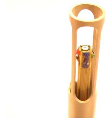
FIGURE 4.19: Physical size of the *Microflown USP-regular* sensor and the configuration of the three orthogonally placed particle velocity sensors and the collocated miniature pressure transducer in their centre can be observed.
