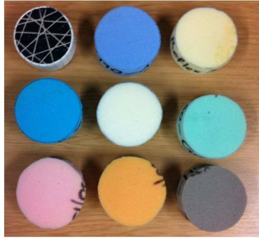
FIGURE 4.1: Sound absorbing samples. Samples are *RX30/080*, *RX33/160*, *RX33/190*, *RX39/200*, *RX41/150*, *RG50/100*, *RG50/135*, *RG50/230* and *needled felt - F1O*.
