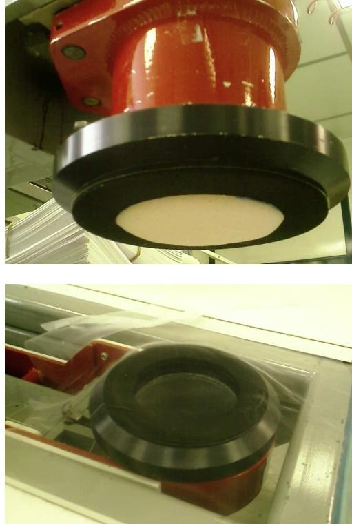
FIGURE 4.5: *Aermacchi* DC-flow rig loaded with porous sample.
