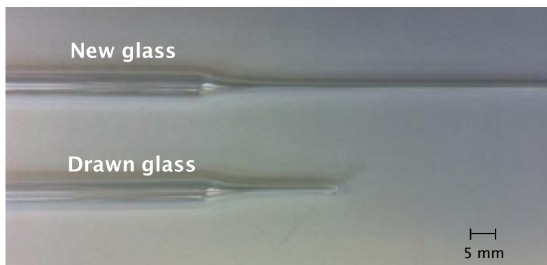
Figure 3-3 Glass pipettes used for the nozzle in the dispensing device.
