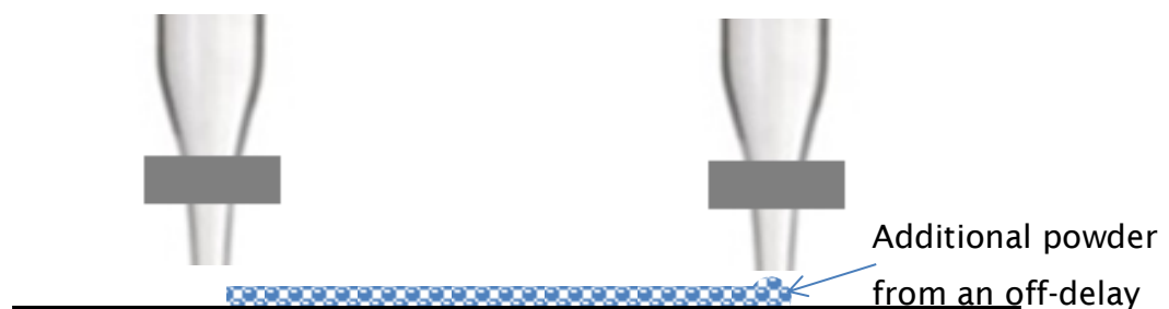
Figure 4-9 The effect of an off-delay time in powder printing.
