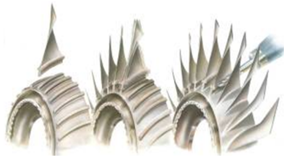
Figure 2.9: Linear Friction Welding. a) Disc and Blade Before LFW, b) LFW Process, and c) Adaptive Milling
