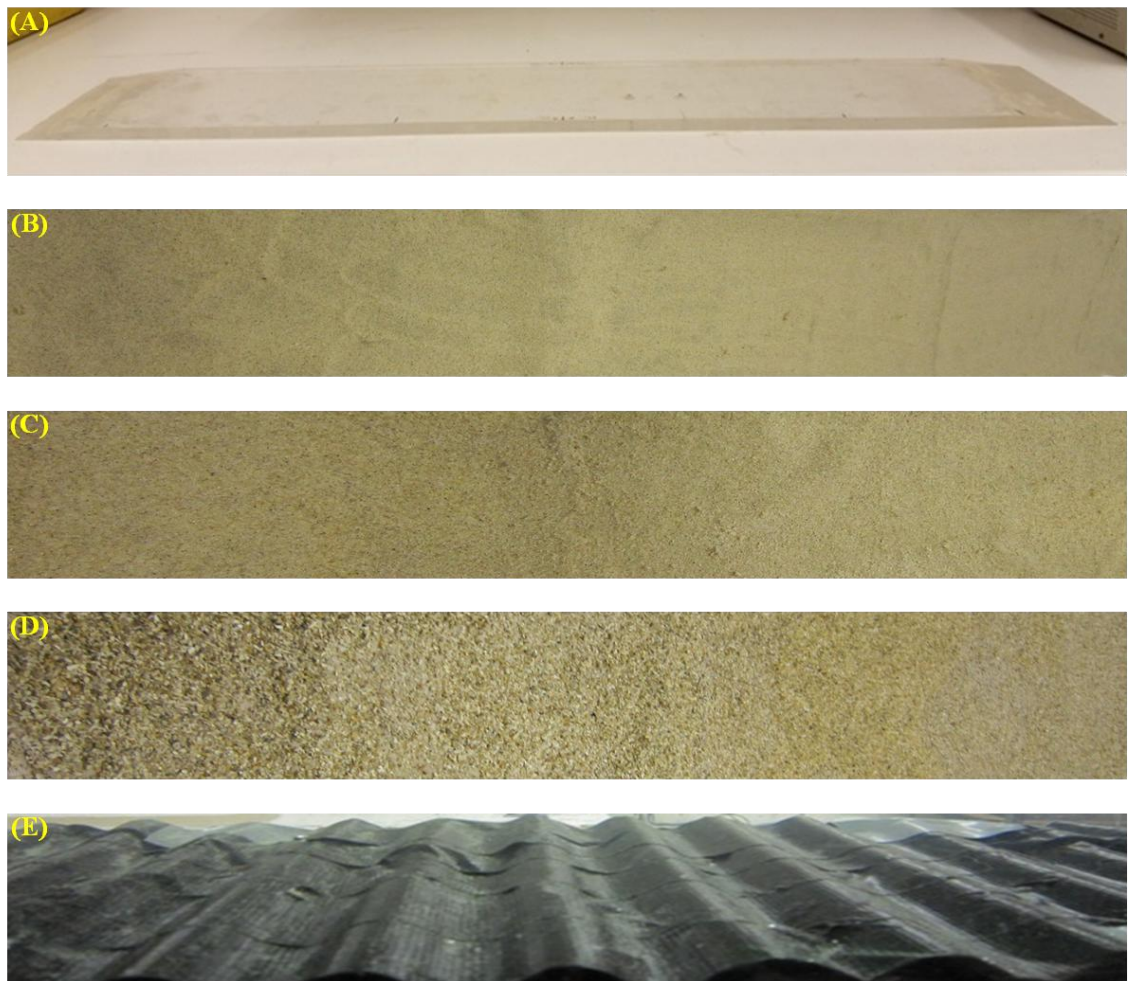
Figure 5.6: (A) Plexiglas smooth 1 m base (B) fine sand (125 \mu m) (C) medium sand (0.25 mm) (D) coarse sand (0.5 mm) and (E) rippled plastic sheet.
