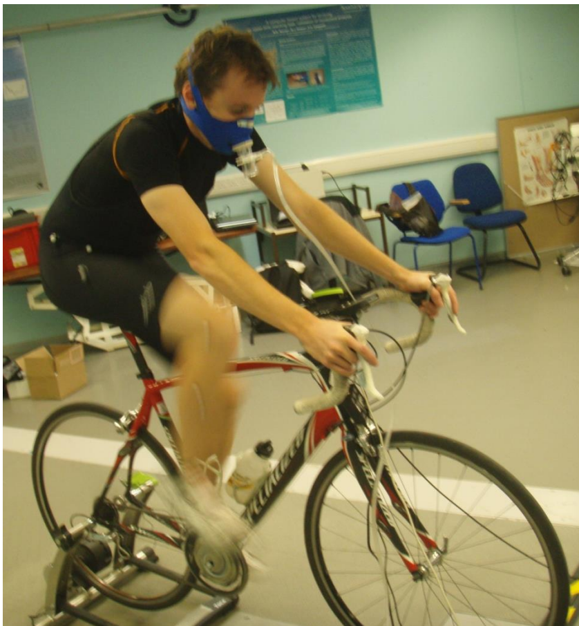
Figure 4-2; Photograph of experimental platform from a data collection session. Bike is mounted on the ergometer with the SRM cranks mounted on the bike. Motion capture markers have been placed on the bike and rider and the rider is wearing a breath analyser mask
