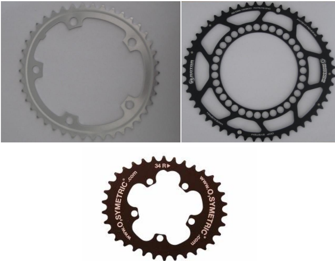
Figure 1-3; Three production non-circular chainrings, from top left going clockwise: Shimano Biopace, Rotor Q-Ring, and O.Symetric Harmonic
