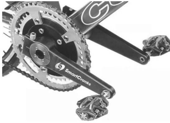
Figure 2-10; SmartCrank training system; both cranks can move independently of each other but only one can drive the chainring at a time
