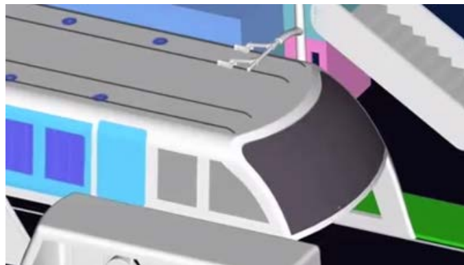
Figure 4-2 Overhead lines for the Straddle Bus
