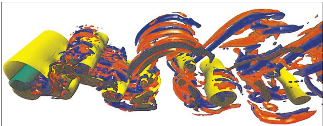
FIGURE 1.13: Instantaneous iso-surfaces of pressure (predominant alignment spanwise) and streamwise vorticity (predominantly streamwise) at Re=556 from 3-D simulation, reproduced by Blackburn et al. [9].
