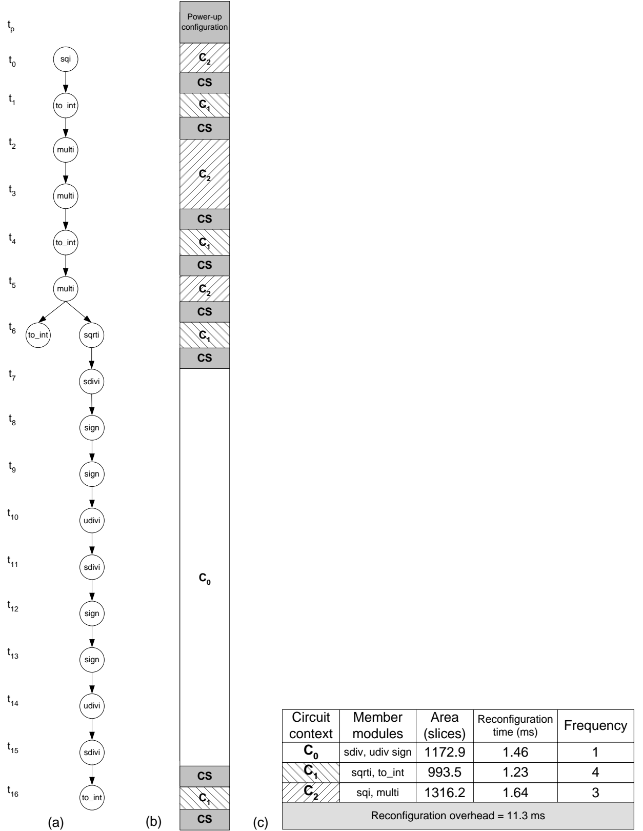
Figure 4.6: Context switching of the partitioned quadratic equation solver.
