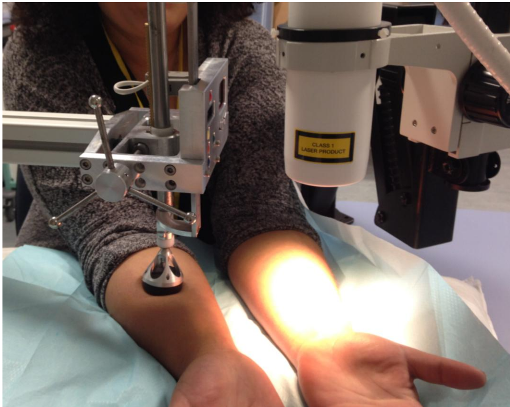
Figure 1. A photograph demonstrating the loading and imaging set-ups. The imaging head of the Fluobeam® 800 (right) was held by an articulated arm, thus allowing easy repositioning to image both arms. The indenter (left) was attached to a secure cantilever beam.
