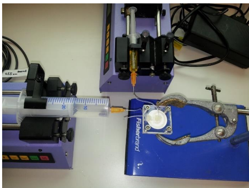
Figure 4.14: Experimental set up for Counter flow arrangement (1) Water supply from a syringe flow rates 10-750 \mu L/min, (2) Sample supply from a syringe, flow rates 0.5-50 \mu L/min and (3) membrane of MWCO-5000Da used to design sandwiched dialysis device.
