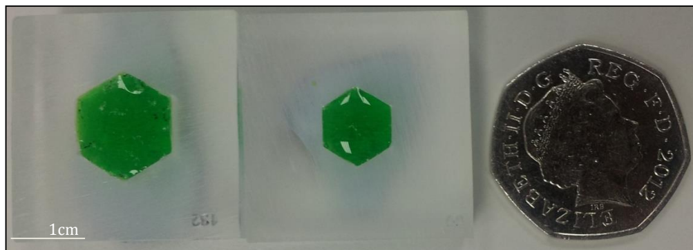
Figure 4.7: Basic dialysis device to check the performance of the membrane. The ultrafiltration membrane is glued to the acrylic. The hexagon has an area of 132mm 2 and 66mm 2 .
