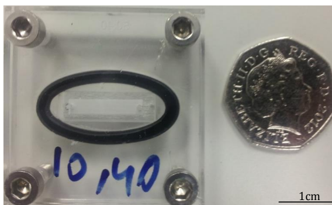
Figure 4.10: Rectangular dialysis setup with 'O' rings to provide tight sealing of the membranes for stop and flow experiment
