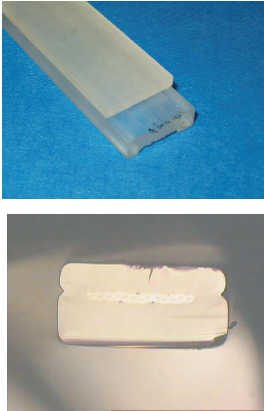
Figure 4.24: Demonstration of a method for fabrication of multiple core in a single fibre. A channel is cut into which caned preforms are inserted, and then covered with a slab of silica. When drawn the fibre is shown to be fused together indicating that two pieces of glass in contact within the furnace will fuse together.
