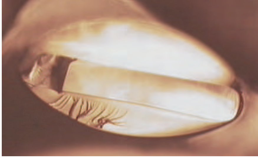
Figure 4.5: Photograph showing the coating of a rectangular fibre. The coating is thin at the corners of the fibre, which leads to structural weakness. The fibre has dimensions of 1.8\text{mm} \times 150\mu\text{m} .
