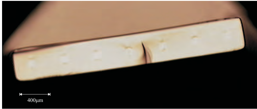
Figure 4.4: A low drawing temperature to maintain the rectangular profile, causes the viscosity of the glass to increase to a point where the air gaps surrounding the inserted core rods are not completely sealed. The fibre has dimensions of 2\text{mm} \times 140\mu\text{m} .
