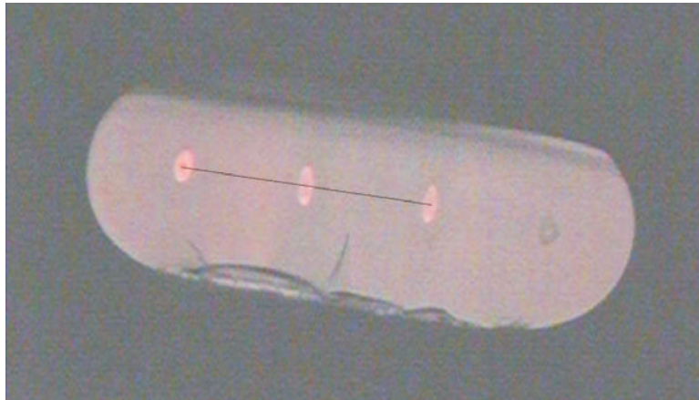
Figure 4.26: A photograph of the end face of the fibre fabricated using the fusing effect of silica in the furnace. The dimensions of the fibre are in a ratio of 3:1 whilst the preform had dimension in the ratio of 4:1. The cores bear evidence to the deformation of the fibre during drawing. The dimensions shown are 1\text{mm} \times 300\mu\text{m}
