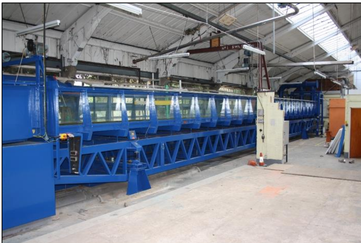
Figure 3.1 Twenty one metre long indoor flume facility at the International Centre for Ecohydraulics Research (ICER) facility, University of Southampton, UK.
