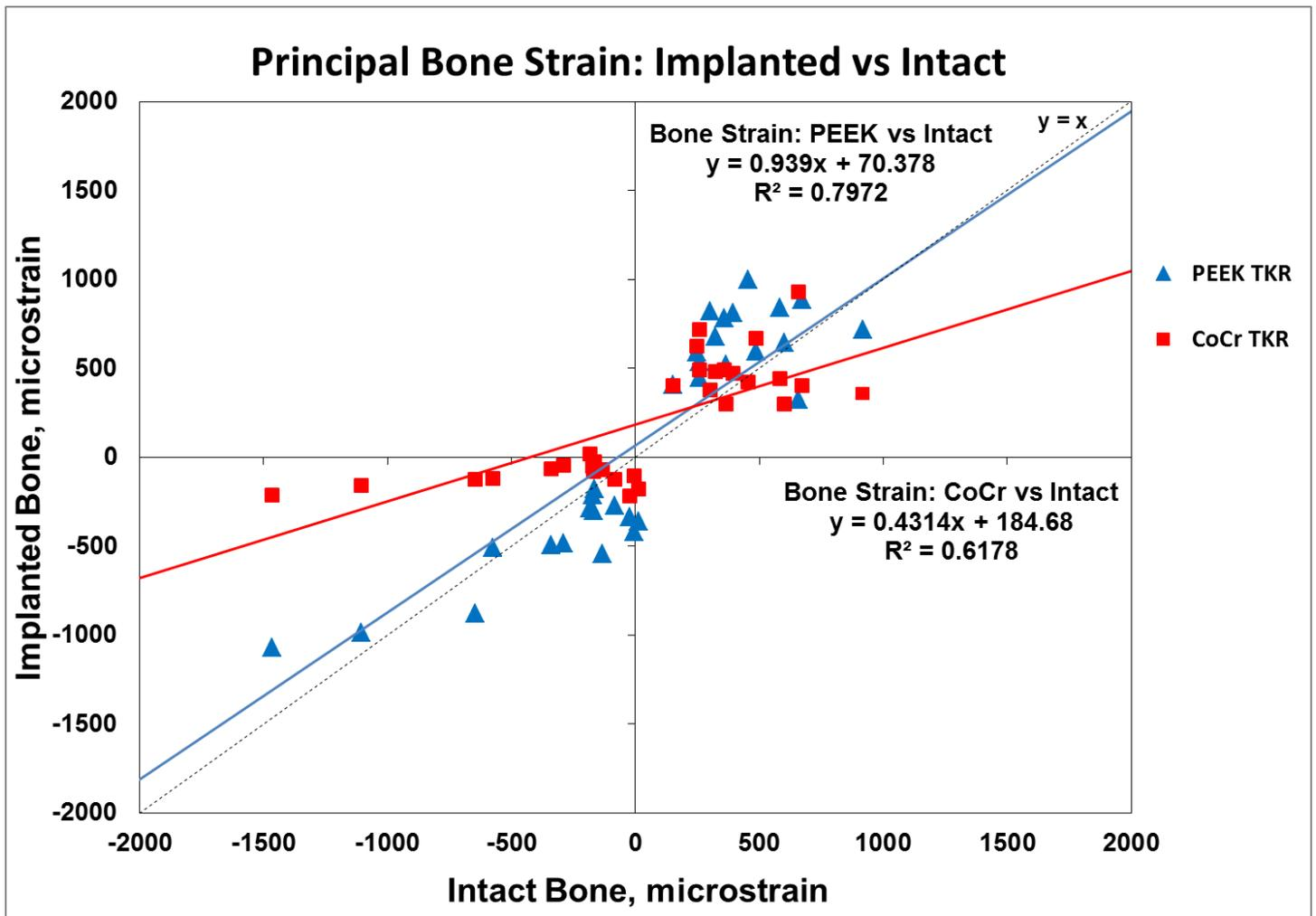
**Fig. 6** A quantitative comparison of principal strain on the intact analog bone surface with corresponding ROIs on the implanted cases showed that there was a large deviation with the CoCr bone model strain compared with the PEEK bone model strain.
