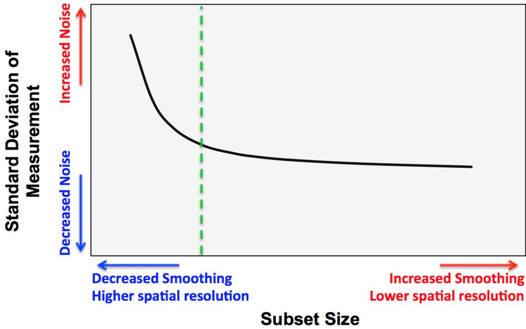
**Fig. 2** The selection of DIC subset size is a tradeoff between noise and smoothing of the data under nominally zero strain conditions (an example curve is shown where the green dashed line represents the subset size that may be optimal).
