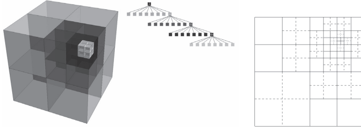
FIG. 1. Leaves of an adaptive 3D MR mesh, left. Sketch of the corresponding octree structure, middle. Leaves (plain) and virtual leaves (dashed) of an adaptive 2D MR mesh, right.
