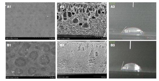
Fig.10 Morphology and the contact angle of PVC/PVB composite membranes (A: the membrane prepared under optimized parameters in the case of using pure water as gelation bath, B: the membrane prepared under optimized parameters in the case of using DMAc as the solute of gelation bath. 1. Suface structure 2. Crosssection structure 3. Contact angle)
