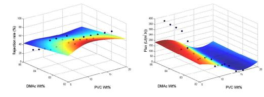
Fig. 7 Training data and fitting curves of rejection rate and flux in the subspace of
