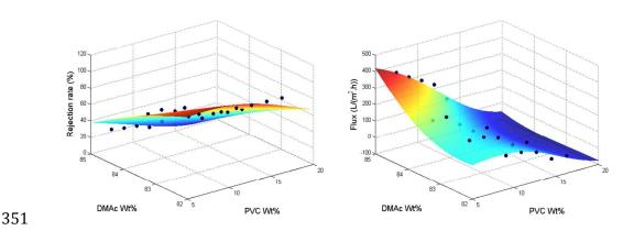
Fig. 8 Training data and fitting curves of rejection rate and flux in the subspace of
