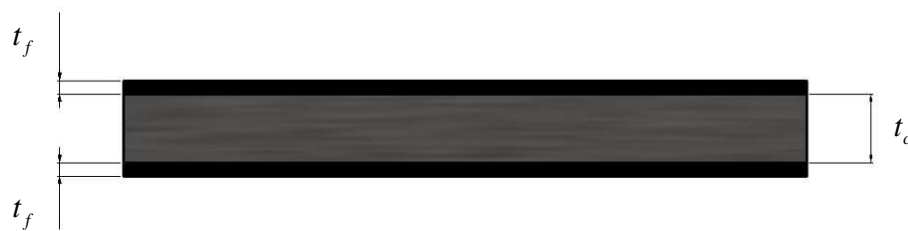
Figure 98 : Schematic Representation of a Sandwich Panel
