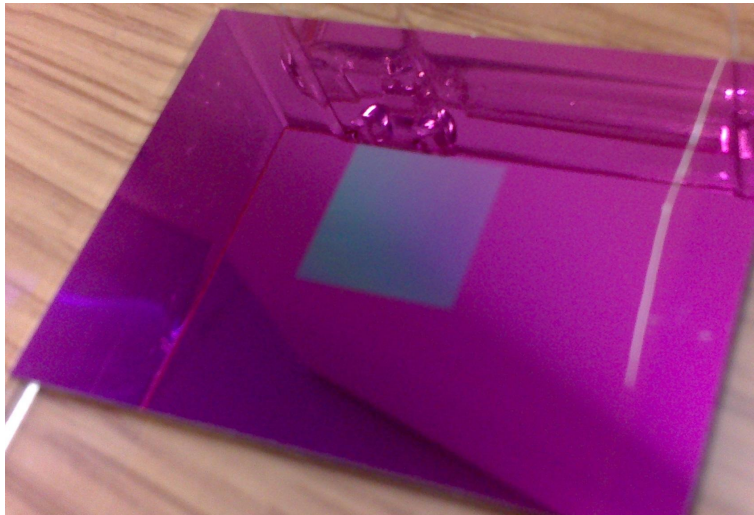
Figure 7.9: 1x1cm Defined 200nm octagonal pattern on silicon substrate
