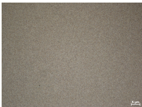
Figure 6.2: 150x optical microscope image of metal-island films on glass
