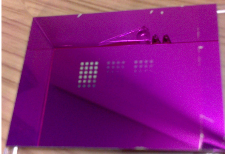
Figure 7.8: 3 x 24 Region dose test patterns on silicon substrate
