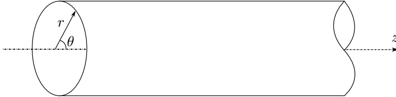
Figure 3.3: Schematic of the cylindrical coordinate system for a clean circular duct.
