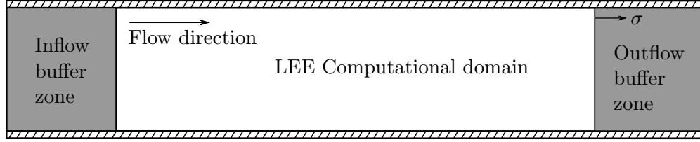
Figure 3.11: A schematic of the buffer zone implementation.
