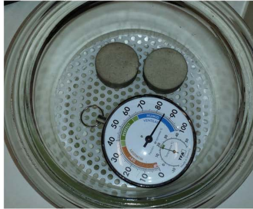
Figure 4.1: a) blank rock (left) and fractured rock (right). b) A schematic of the synthetic rock containing aligned fractures c) rock samples in vacuum desiccator containing saturated salt solution, and a hygrometer to verify the relative humidity.
