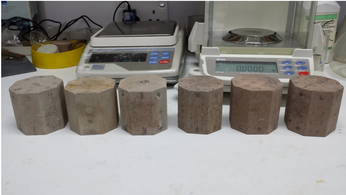
Figure 6.3: Octagonal sandstone samples. First three from the left are blank samples and the other three samples contain PVA discs (fractured samples).
