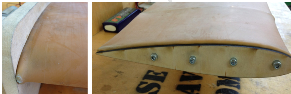
Fig. 9. Skin-ribs clamping mechanism.
