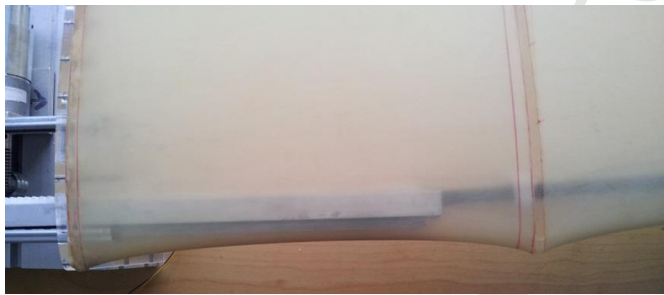
Fig. 11. Poisson's contraction of the skin when fully extended.
