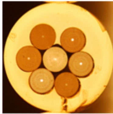
Fig. 3.1 Microscope image of a Er-doped 7-MEF showing the arrangement of 7 fibre-elements in the high index coating
