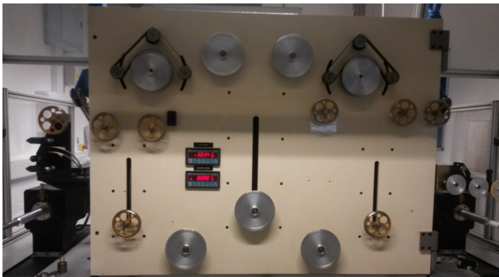
Fig. 5.9 Proof-test and rewinding machine
