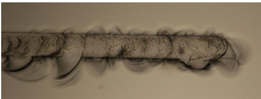
Figure 90. Microscope image of 50 \mu\text{m} wide groove.
