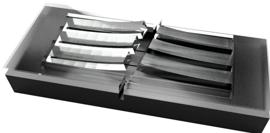
Figure 53. Shows a 3D visualization showing the concept of dual opposing cantilevers machined into silica-on-silicon. Each cantilever contains an optical waveguide. The cantilevers are produced using dicing technology and etching away silicon to release the silica structures.
