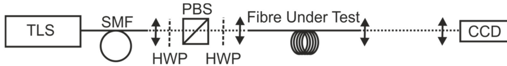
Fig. 2. Spatial and spectral ( S^2 ) imaging setup. TLS: Tunable Laser Source, SMF: Single Mode Fiber, HWP: Half-wave plate, PBS: Polarizing beam splitter, CCD: InGaAs camera, Lenses shown by double headed arrows.
