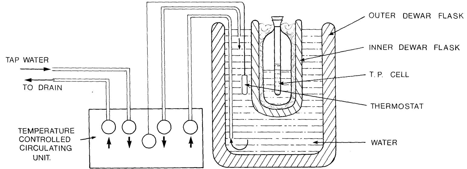
FIG. 1 ARRANGEMENT FOR KEEPING THE  $26.8685^{\circ}\text{C}$  AND THE  $36.3241^{\circ}\text{C}$  TRIPLE POINT CELLS FOR LONG PERIODS.
