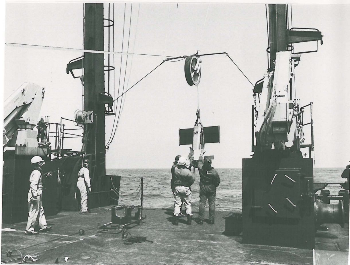
Figure 1:- SeaSoar and Winch as deployed during Vivaldi '91 Top picture shows winch holding 750m of faired cable partially paid out. Lower picture shows SeaSoar hanging beneath the "A" frame prior to deployment
