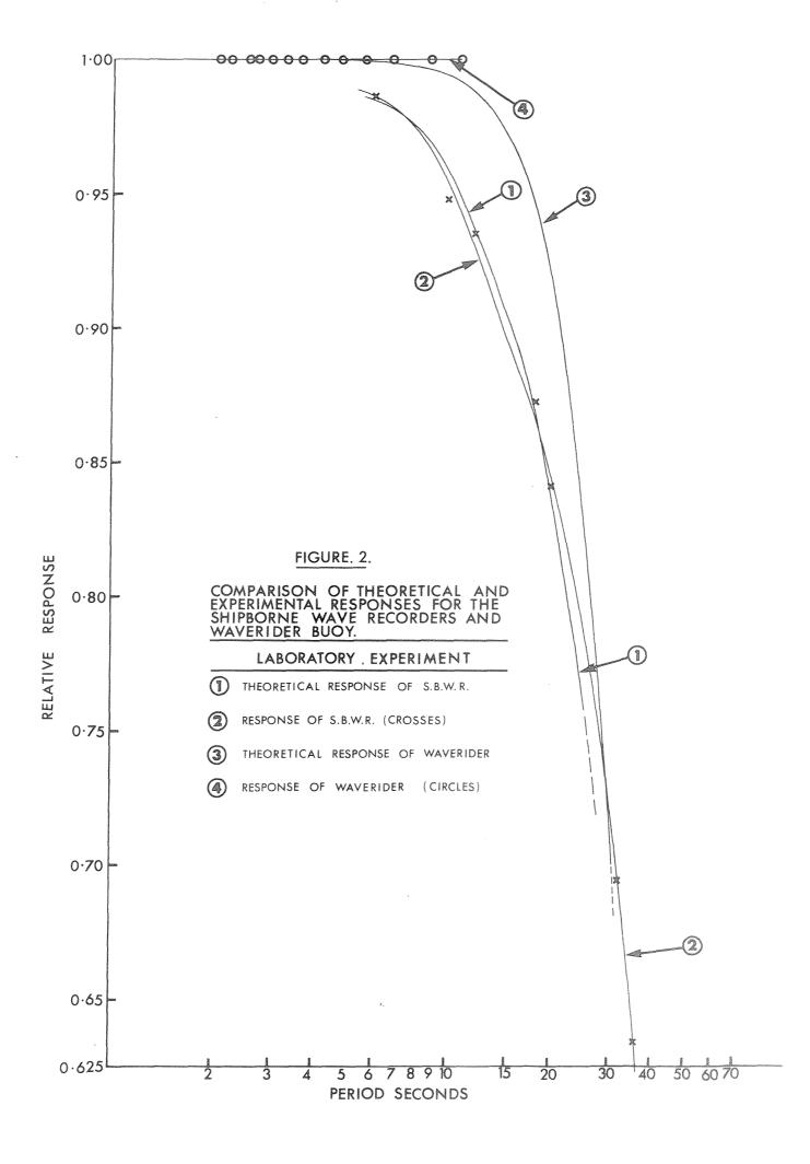
The period of rotation can be varied from 2 seconds to 15 seconds approximately, although the I.O.S. buoy was tested rigorously only up to 10.8 seconds.
