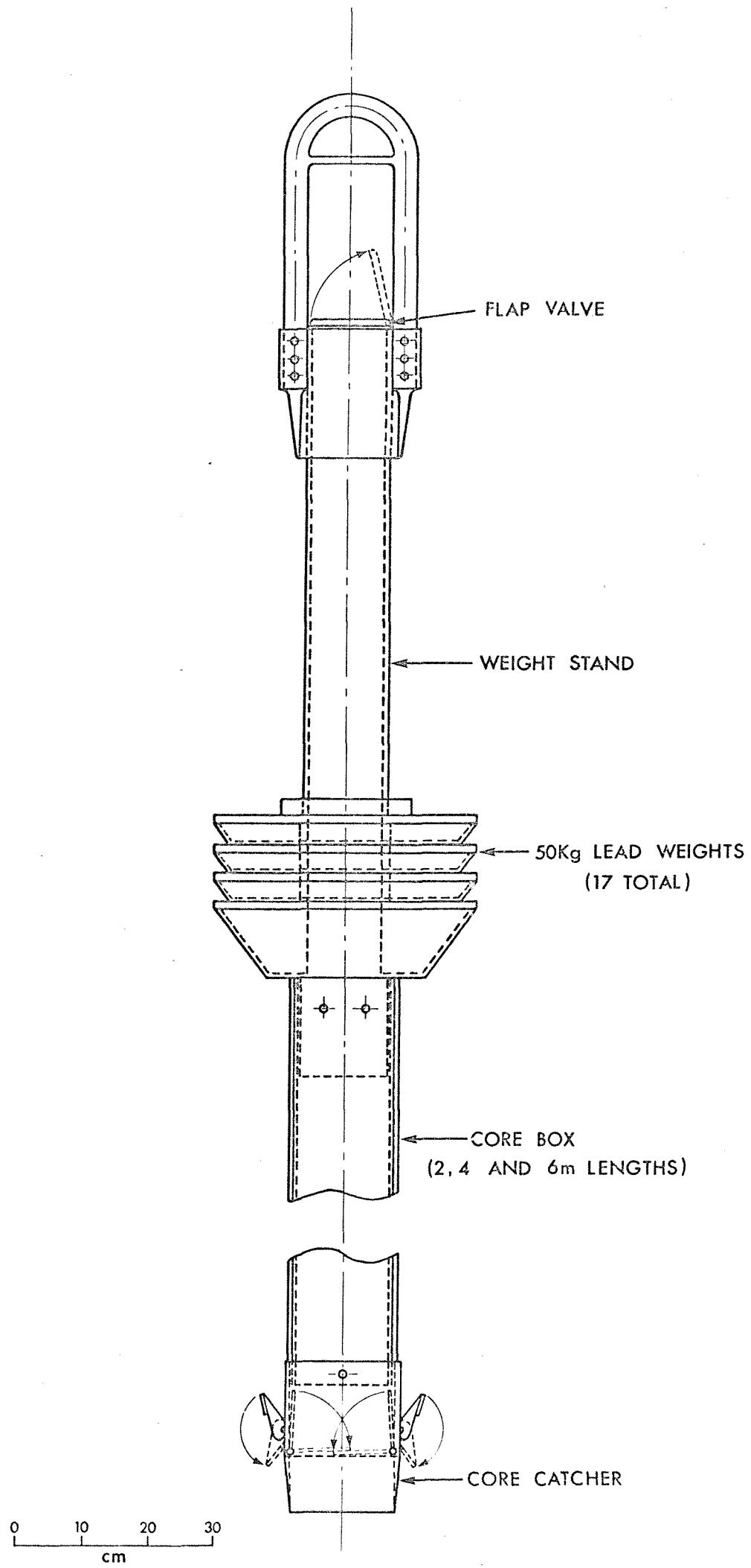
Fig. 2a Assembled corer in deck cradle on R.R.S. Discovery.
