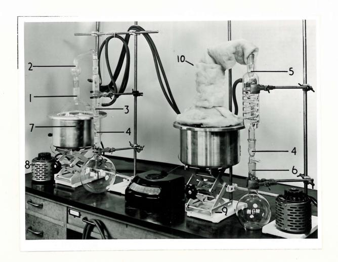
Figure One: Pyrex stills for stages one and two of distillation
