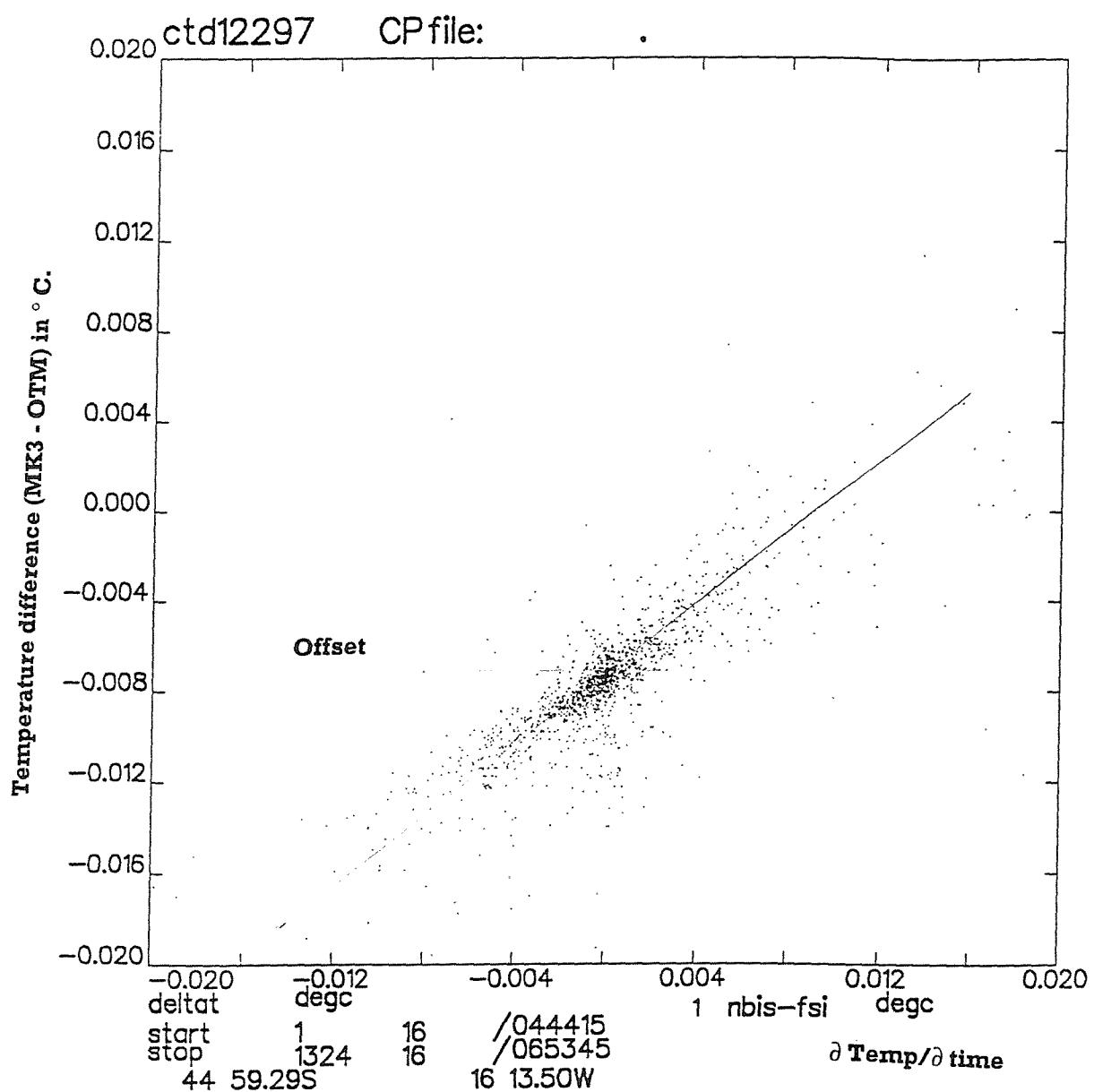
Figure 6. Scatter Plot of MK3 and OTM temperature difference.
