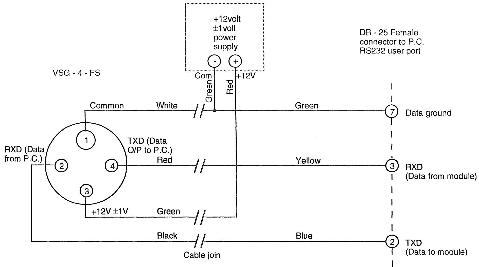
Figure 1 Cable connection - P.C. to OTM
