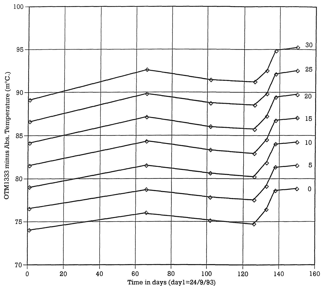
Fig. 3 - 84 Day Temperature difference with Time
