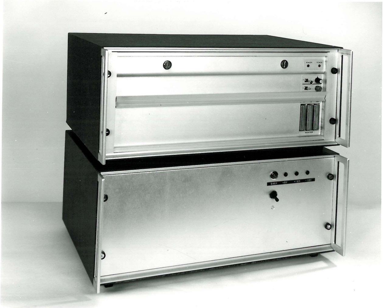
Fig. 15 Memory cabinet (top) and power supply cabinet (bottom).
