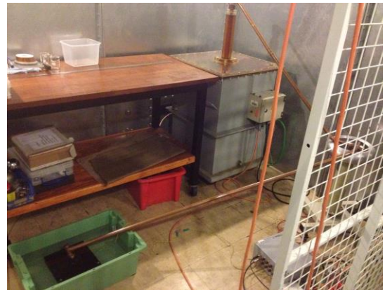
Figure 3-10: Full setup of multiple samples stressing experiment.
