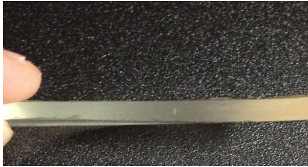
Figure 3-2: Interface of two combined pieces of epoxy resin
