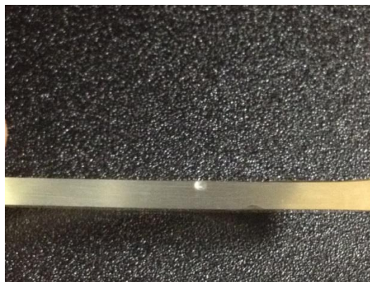
Figure 3-3: bubble injected early flows up due to buoyancy force
